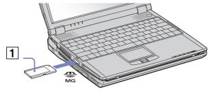
Hold the Memory Stick<sup>TM</sup> with the arrow pointing in the correct direction when you insert it into the slot. To avoid damaging the computer or the Memory Stick<sup>TM</sup>, do not force the Memory Stick<sup>TM</sup> into the slot if it does not insert smoothly.
